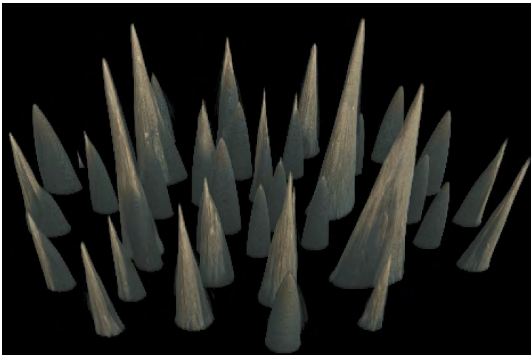
Fig. 2. Nano-micro composite fluid (CMF) in non-uniform magnetic field: formation of spikes similar to Rosensweig instabilities in case of ferrofluids
