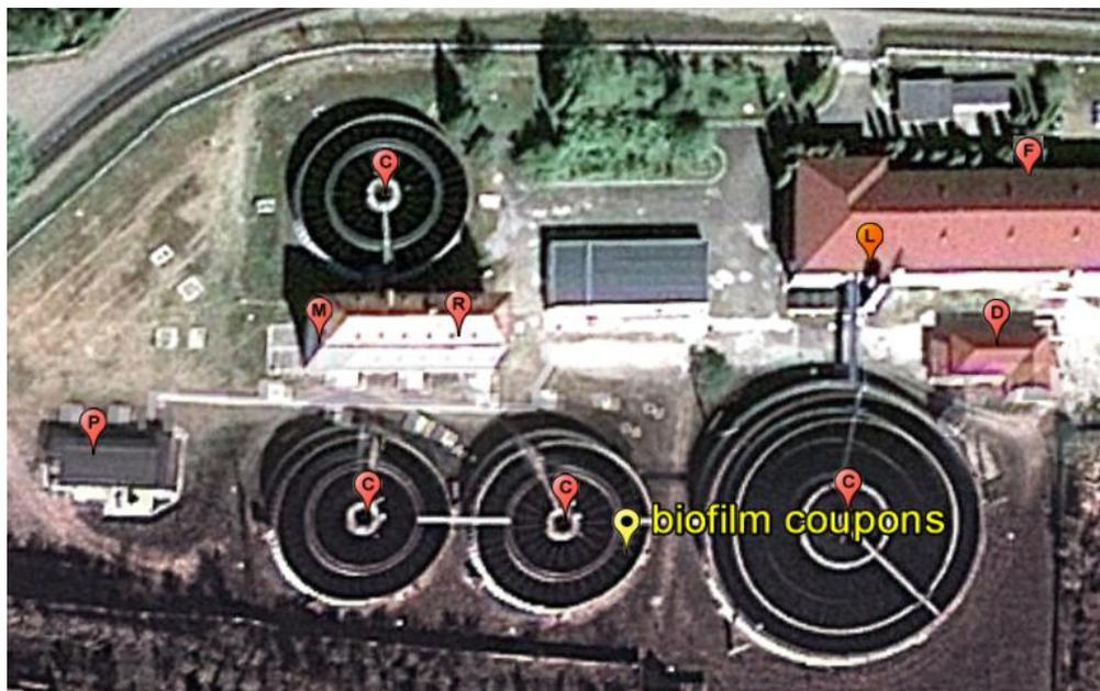
**Figure 1.** The drinking water treatment plant of Cluj with the position of the immersed polypropylene coupons. M – microstraining; P – prechlorination; R – reagents addition for coagulation and flocculation; C – clarification; F – rapid sand filtration; D – final disinfection by chlorination; L – laboratory.
