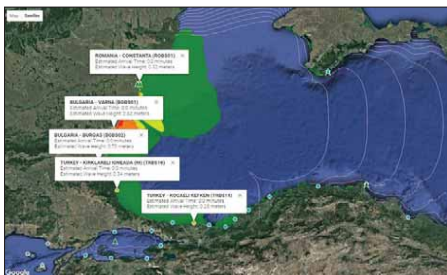
Fig. 4. Map with the estimated wave heights for certain locations for the worst case scenario (M 8, depth 5 km) using TRIDEC software
