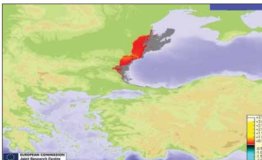
Fig. 9. Maximum wave heights for the moderate scenario (M 7.5, depth 10 km) using TAT software
