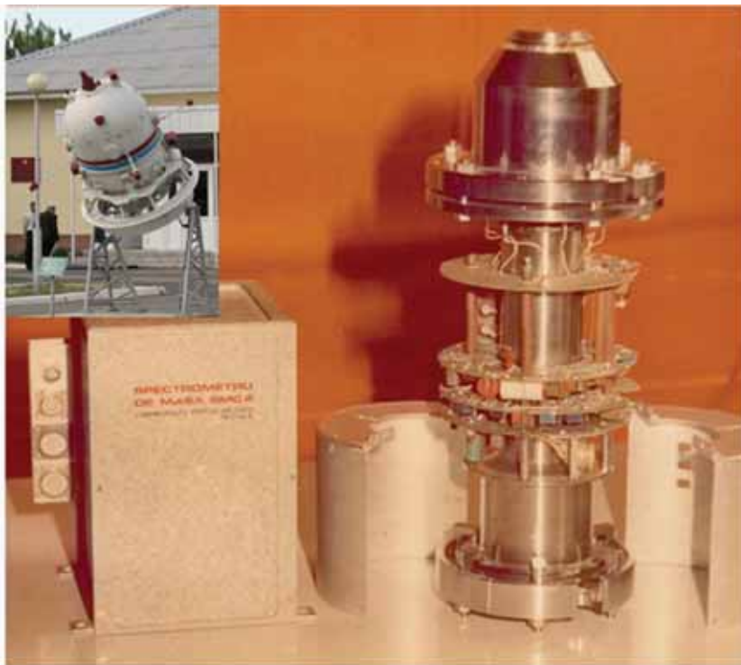
Fig. 7. Mass Spectrometer QMS-3. The electronic block (bottom left), the container (top left) and the mechanical part of the QMS-3 (right) on which is installed the radio frequency generator and the electrometer.
