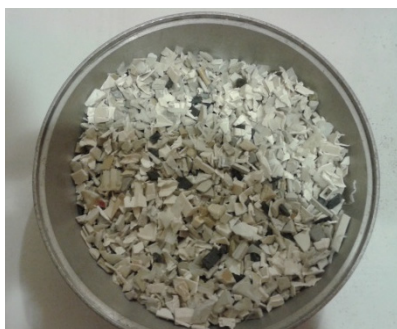
Fig.1. WEEE plastic minced photo: Antoanela Popovici
