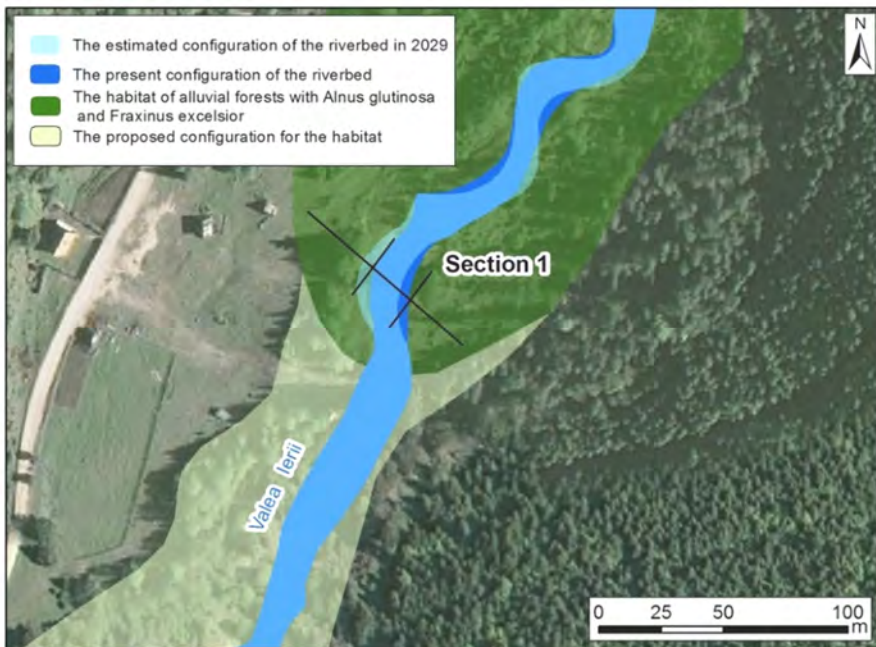
Fig. 3. The simulation of the configuration for Valea Ierii river and alluvial forests habitat in Section 1
