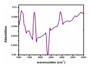
Figure 5. Typical FTIR absorbance spectra of the diamond films grown on S<sub>2</sub>
