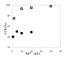
Figure 3. The evolution of the electrochemical parameters, CCE and SD, in 0.5 M  $(\Box)$  and 2 M H<sub>2</sub>SO<sub>4</sub>  $(\bullet)$  for different concentrations of Zn<sup>2+</sup>, i =217 A/m<sup>2</sup>
