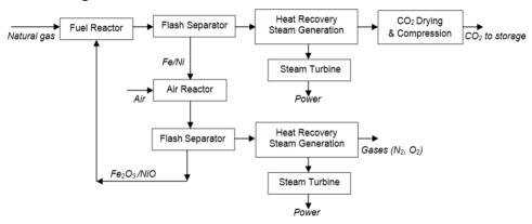
**Figure 2.** Chemical looping combustion for power generation
