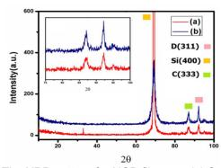
Figure 4. The XRD pattern for NCD films on: (a) S<sub>1</sub> and (b) S<sub>2</sub>
