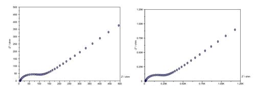
**Figure 1.** Impedance spectra of  $0.5 \cdot 10^{-3}$  M potassium ferro/ferricyanide at unmodified (left) and clay modified SPE (right) in 0.25M KCl
