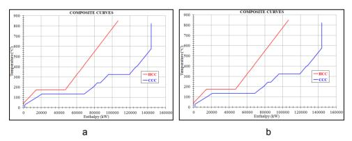
**Figure 3.** Composite curves for heat recovery from CO<sub>2</sub> stream (fuel reactor) a. CLC using ferric oxide; b. CLC using nickel oxide
