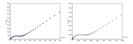
**Figure 2.** Impedance spectra of 0.5·10<sup>-3</sup> M potassium ferro/ferricyanide at unmodified SPE (left) and ZPG modified SPE (right) in 0.25 M KCl
