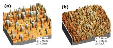
**Figure 2.** Three dimensional AFM images of silicon coated by (a) Gold and (b) silver nanoparticles.
