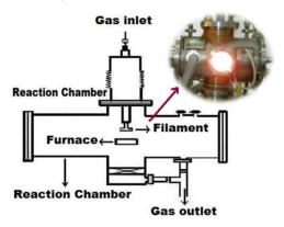
Figure 7. Schematic diagram of the HFCVD system
