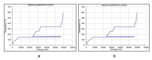
**Figure 4.** Grand composite curve for heat recovery from CO<sub>2</sub> stream (fuel reactor) a. CLC using ferric oxide; b. CLC using nickel oxide
