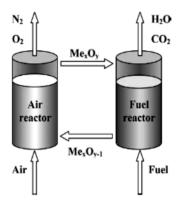
Figure 1. Chemical looping combustion (CLC)
