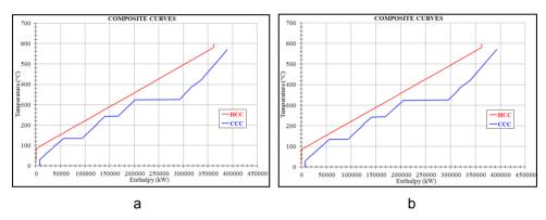
**Figure 5.** Composite curves for heat recovery from spent air stream (air reactor) a. CLC using ferric oxide; b. CLC using nickel oxide
