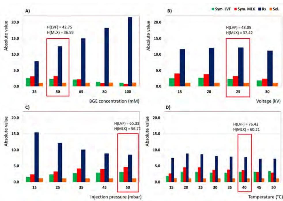
**Figure 3.** Variation of symmetry, resolution and selectivity of analytes signals in terms of **A)** BGE concentration, **B)** voltage, **C)** injection pressure and **D)** temperature (*Sym.* – symmetry, *Rs* – resolution, *Sel.* – selectivity, *H* – height of peak).
