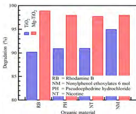
**Figure 9.** The degradation optimum conditions of the organic pollutants using pure TiO<sub>2</sub> and Mg-doped TiO<sub>2</sub>.
