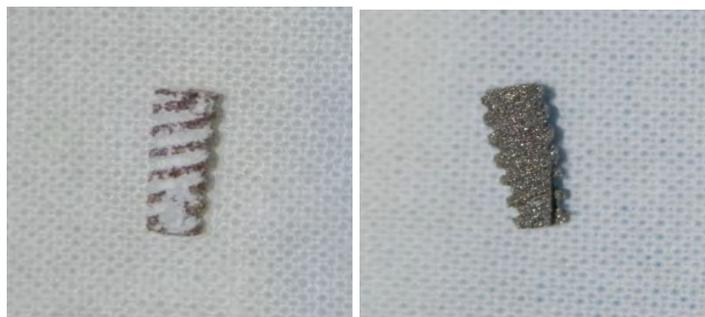
**Figure 6.** a) Ti<sub>6</sub>Al<sub>7</sub>Nb implant coated with HA; b) Ti<sub>6</sub>Al<sub>7</sub>Nb implant coated with SiO<sub>2</sub>-TiO<sub>2</sub>
