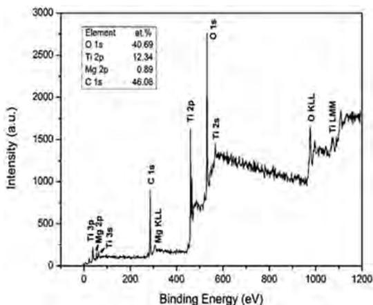
**Figure 3.** XPS survey spectrum for 1.5 at.% Mg-doped TiO<sub>2</sub> nanoparticles, the inset shows the atomic ratio of the elements.
