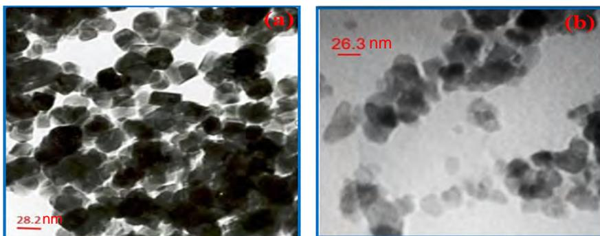
**Figure 2.** Typical TEM micrographs for undoped (a) and 1.5 at.% Mg-doped TiO<sub>2</sub> (b) nanoparticles.
