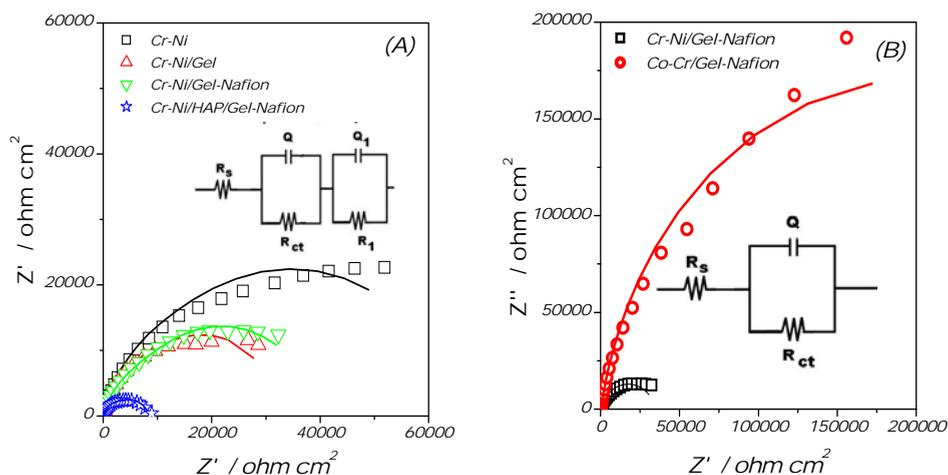
**Figure 2.** Nyquist diagram of different Cr-Ni modified electrode (see inset) (A) and Alloy/Gel-Nafion electrode (B) in artificial saliva solution of pH 7 recorded at OCP after 1 h of stabilisation. Experimental conditions: frequencies, 10 kHz - 10 mHz; amplitude, 0.1 V; room temperature. The line corresponds to the fitting curve of the experimental data using the  $R_s(QR_{ct})(Q_1R_1)$  (A) and the simplified Randles circuit model  $R_s(QR_{ct})$  (B) (see insets).
