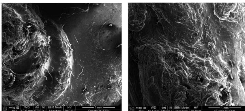
**Figure 1.** SEM at 40X magnification for the bone-implant area Ti<sub>6</sub>Al<sub>7</sub>Nb - SiO<sub>2</sub>-TiO<sub>2</sub> (left) and Ti<sub>6</sub>Al<sub>7</sub>Nb – HA (right).
