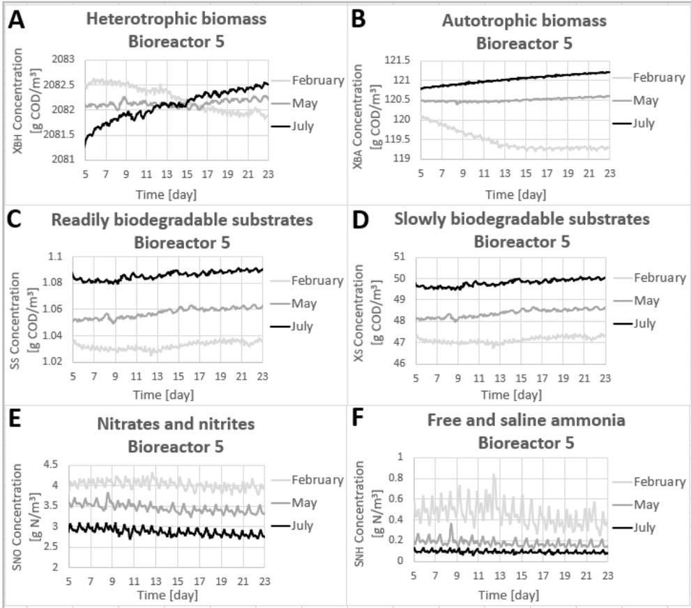
**Figure 4.** The influent temperature effects on the concentrations in the last aerated bioreactor, as response to the three influent temperature changing profiles:
