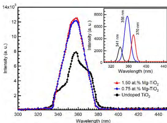
**Figure 4.** Photoluminescence spectra for pure and 1.5 at.% Mg-doped TiO<sub>2</sub> nanoparticles.
