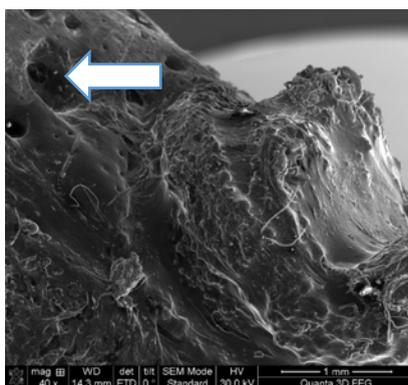
**Figure 2.** SEM at 40X magnification for the bone-implant area Ti<sub>6</sub>Al<sub>7</sub>Nb. Lacunar areas in the bone surrounding the implant (white arrow).
