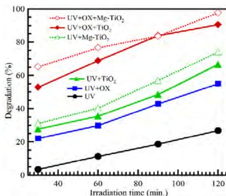
**Figure 7.** Degradation of pseudoephedrine hydrochloride in aqueous solutions: conditions are, pseudoephedrine hydrochloride concentration = 10 mg L<sup>-1</sup>, pure TiO<sub>2</sub> = 0.28 g L<sup>-1</sup>, Mg-doped TiO<sub>2</sub> = 0.28 g L<sup>-1</sup>, OX (H<sub>2</sub>O<sub>2</sub>) = 5 mM, pH = 6, V = 25 mL.
