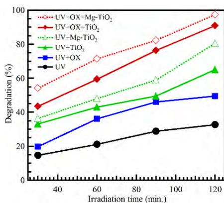
**Figure 6.** Degradation of nonylphenol ethoxylates in aqueous solutions: conditions are: nonylphenol ethoxylates  $6 \text{ mol}$  concentration =  $20 \text{ mg L}^{-1}$ , pure  $\text{TiO}_2 = 0.28 \text{ g L}^{-1}$ , Mg-doped  $\text{TiO}_2 = 0.28 \text{ g L}^{-1}$ , OX ( $\text{H}_2\text{O}_2$ ) =  $1 \text{ mM}$ ,  $\text{pH} = 6$ ,  $V = 25 \text{ mL}$ .
