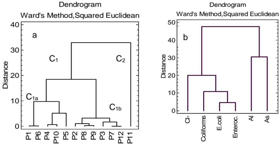
**Figure 4.** Cluster analysis of groundwater samples from Seini: a) Clusters of groundwater samples based on their microbiological characteristics (Coliform bacteria, E. coli bacteria and intestinal enterococci); b) Cluster analysis of similarities between microbiological characteristics and the studied chemical parameters (Cl<sup>-</sup>, As and Al concentrations)
