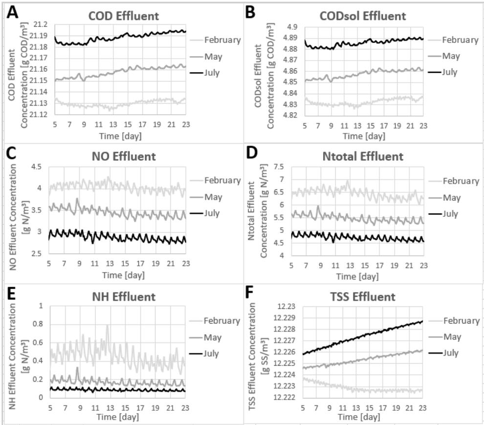
**Figure 3.** The influent temperature dynamic effects on the effluent concentrations, as response to the three influent temperature changing profiles: A. Total COD, B. Soluble COD, C. Nitrates and nitrites, D. Total nitrogen, E. Ammonia, F. Total suspended solids
