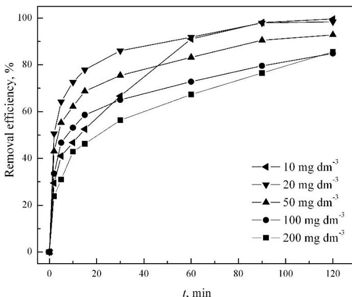
**Figure 5.** Effects of initial Cu(II) concentration on removal Cu(II) by INN (initial Cu(II) concentration  $10.0$ - $200.0 \text{ mg dm}^{-3}$ , temp.  $20 \pm 0.5^\circ\text{C}$ , pH  $5.0 \pm 0.1$ , biosorbent dose  $4.0 \text{ g dm}^{-3}$ )
