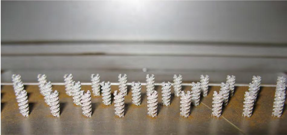
**Figure 4.** Final shape of Ti<sub>6</sub>Al<sub>7</sub>Nb implants after SLM, before the coating process
