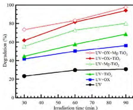
**Figure 8.** Degradation of nicotine in aqueous solutions: conditions are, nicotine concentration = 20 mg L<sup>-1</sup>, pure TiO<sub>2</sub> = 0.28 g L<sup>-1</sup>, Mg-doped TiO<sub>2</sub> = 0.20 g L<sup>-1</sup>, OX (K<sub>2</sub>S<sub>2</sub>O<sub>8</sub>) = 3 mM, pH = 7, V = 25 mL.
