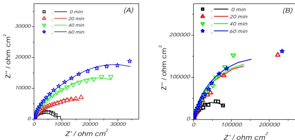
**Figure 3.** Nyquist diagram of Cr-Ni/HAP/Gel-Nafion (A) and Co-Cr/HAP/Gel-Nafion (B) electrode at different time (see inset) of exposure to artificial saliva solution of pH 7 recorded at OCP, after 1 h of stabilisation. Experimental conditions: see Fig 2.
