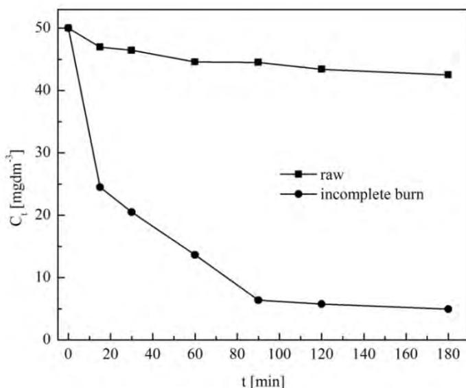
**Figure 4.** Effect of contact time on removal Cu(II) by raw nettle and nettle after incomplete incineration (initial Cu(II) concentration 50 mg dm<sup>-3</sup>, temp. 20±0.5 °C, pH 5.0±0.1, biosorbent dose 4.0 g dm<sup>-3</sup>)
