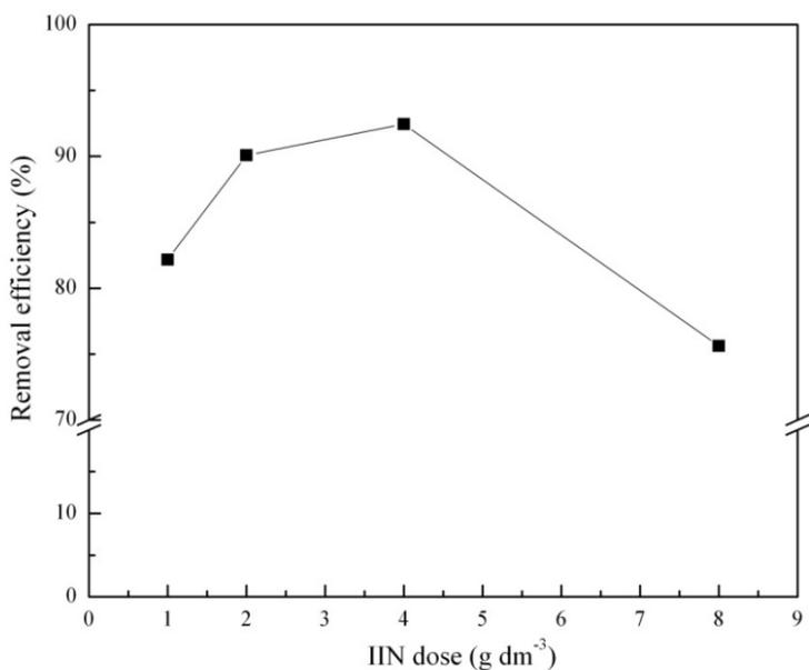
**Figure 6.** Effect of biosorbent dosage in a removal of Cu(II) ions (initial Cu(II) concentration 50.0 mg dm<sup>-3</sup>, temp. 20±0.5 °C, pH 5.0±0.1)
