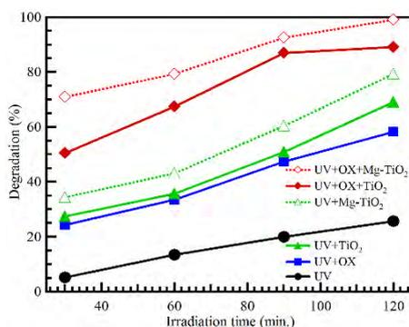
**Figure 5.** Degradation of rhodamine B in aqueous solutions: conditions are, rhodamine B concentration =  $10 \text{ mg L}^{-1}$ , pure  $\text{TiO}_2 = 0.28 \text{ g L}^{-1}$ , Mg-doped  $\text{TiO}_2 = 0.20 \text{ g L}^{-1}$ , OX ( $\text{K}_2\text{S}_2\text{O}_8$ ) =  $3 \text{ mM}$ ,  $\text{pH} = 10$ ,  $V = 25 \text{ mL}$ .
