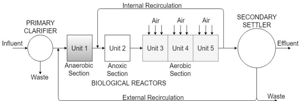
**Figure 1.** The A<sup>2</sup>O configuration of the investigated municipal WWTP
