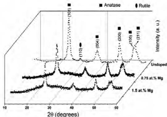
**Figure 1.** X-ray patterns of pure and Mg-doped TiO<sub>2</sub> nanoparticles.
